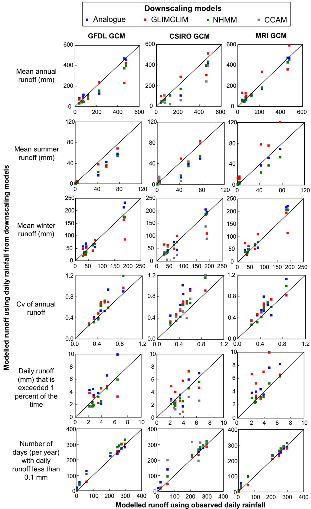
**Fig. 6.** Comparison of runoff characteristics from SIMHYD rainfall–runoff modelling using daily rainfall from the four downscaling models with the runoff modelled using observed daily rainfall over the 1986–2000 period.
