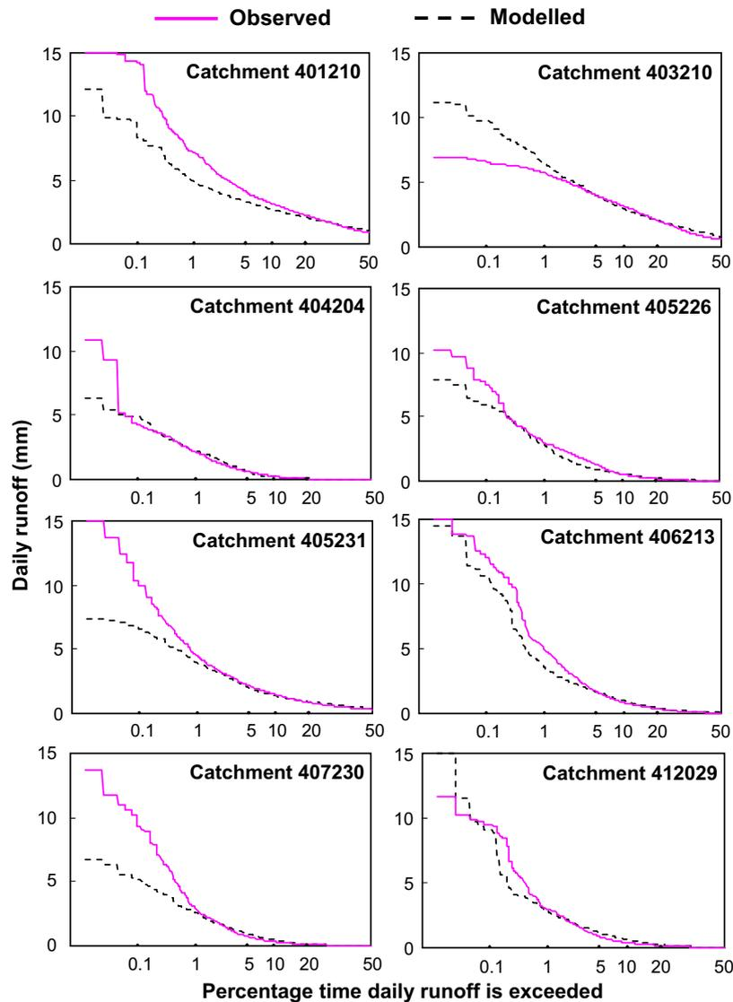
Fig. 4. Comparison of modelled (by the SIMHYD rainfall–runoff model) and observed daily runoff distributions over the 1986–2000 period.
