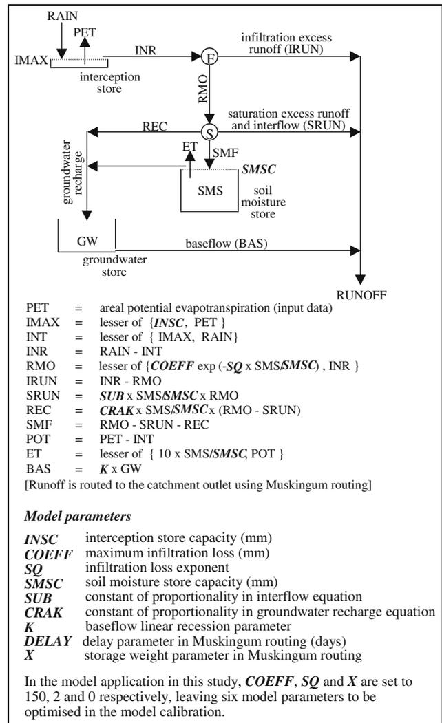
Fig. 2. Structure of the daily lumped conceptual rainfall-runoff model SIMHYD.
