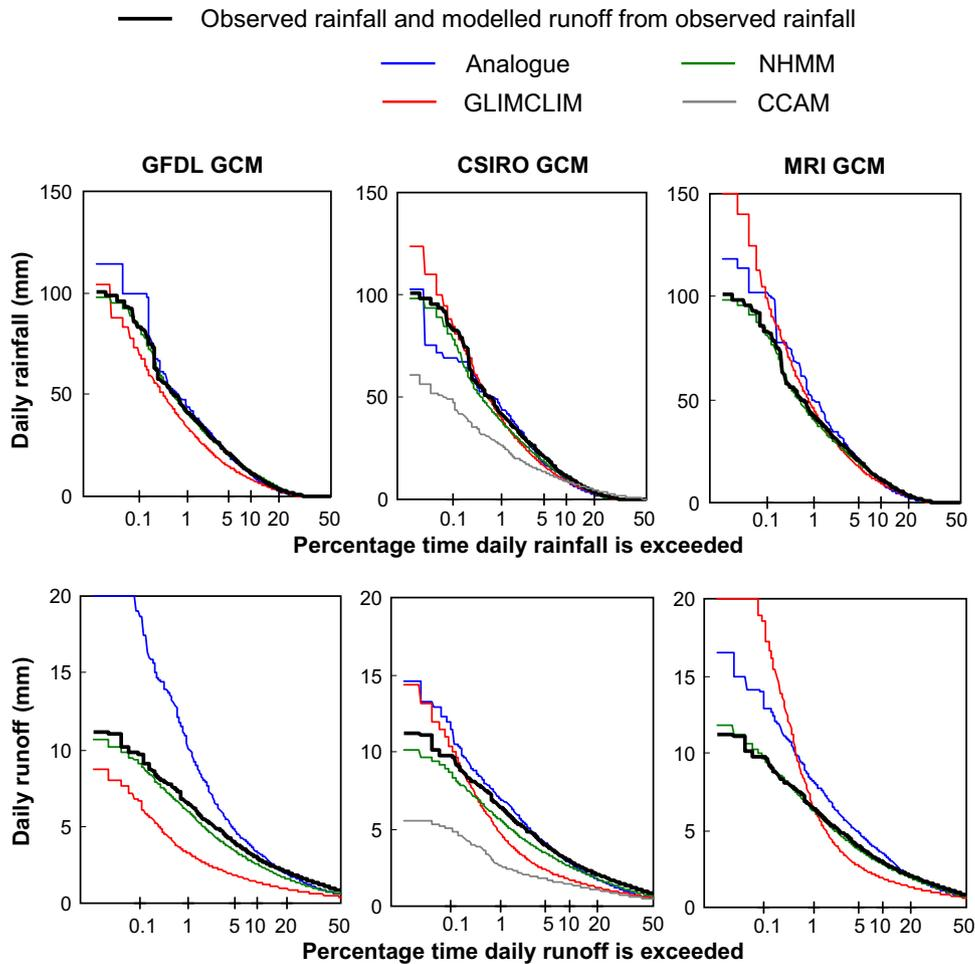
Fig. 7. Comparison of modelled and observed daily rainfall distributions and comparison of daily runoff distributions modelled using downscaled rainfall and using observed rainfall for Catchment 403210.
