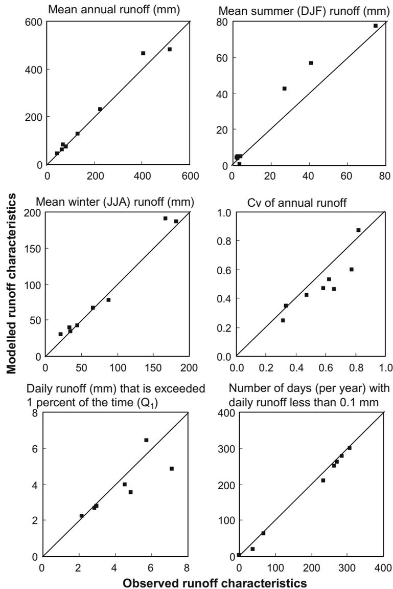
**Fig. 3.** Comparison of modelled (by the SIMHYD rainfall–runoff model) and observed runoff characteristics over the 1986–2000 period (one point for each of the eight catchments).
