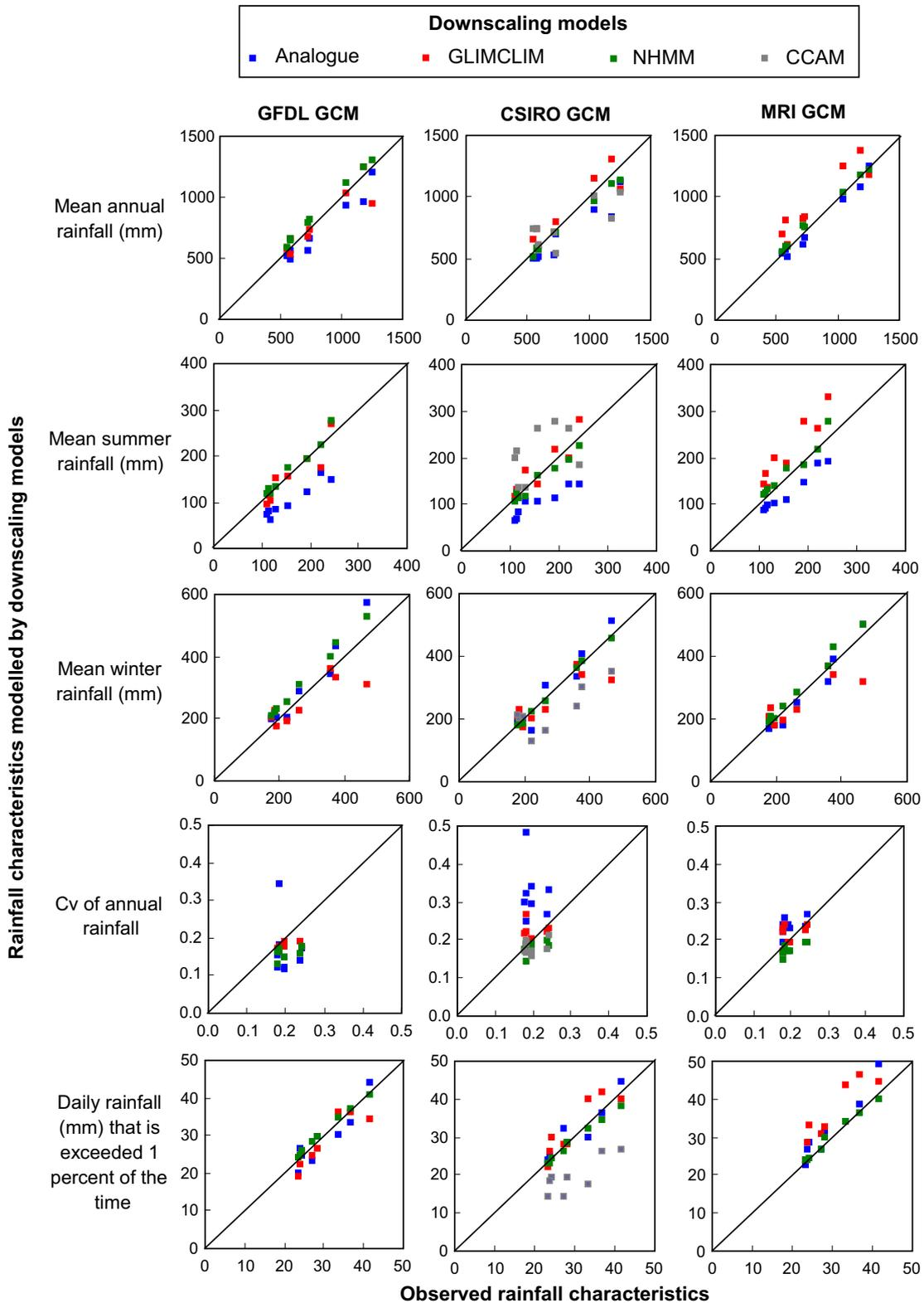
**Fig. 5.** Comparison of rainfall characteristics downscaled from three GCMs by the four downscaling models with the observed rainfall characteristics over the 1986–2000 period.
