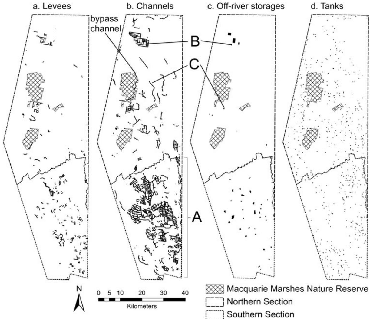
Figure 2. Distribution of (a) levees, (b) channels, (c) off-river storage units and (d) tanks on original Macquarie floodplain including the Nature Reserve within the study area, divided into the Northern and Southern Section. Most irrigation development is in the Southern Section (A), with the exception of two other clusters of irrigation development, B and C in the Northern Section. The 18.5 km bypass channel circumvents wetlands in the Northern Nature Reserve for downstream supply
