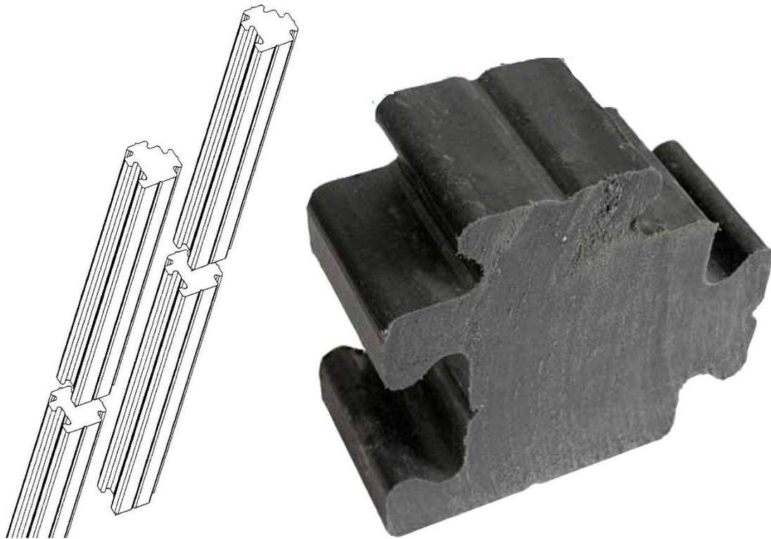
Figure 2: Drawing of a plastic pile (left) and close up image of a cross-section of a portion of a two-dimensional interlocking plastic pile (right), as might be used to construct a barrier across the Coorong. These plastic piles are made from recycled plastic. For more details on this system and their use in constructing barriers visit: <http://www.vonmac.com.au>
